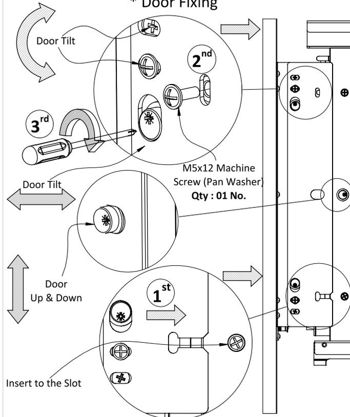
**Step No: 08** \* Door Connecting Arm Fixing
